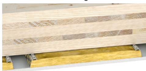
CLT/X-LAM suspended ceiling
